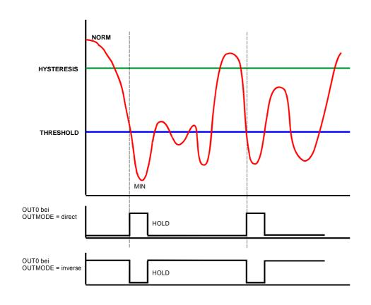
When the sensor detects an edge (NORM VALUE drops below THRESHOLD), a search for the minimum NORM VALUE is performed until the end of the DEAD TIME (TRIGGER=CONT) or the ACTIVE TIME (TRIGGER=EXT) and during HOLD. This minimum value is stored in a 16-value JUMP-BUFFER that can be read out with the GETBUFF software button.
